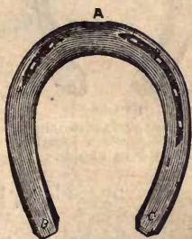
(No. 22.) The ground surface of a common shoe, with lo- cation of nail-holes.
